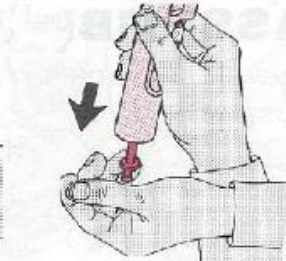
(10) Drop firing pin out to the rear of bolt carrier.
